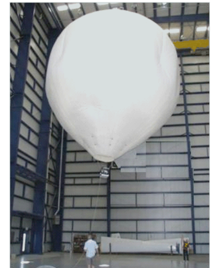
Indoor propane-heated flight of 9 m prototype montgolfière balloon
