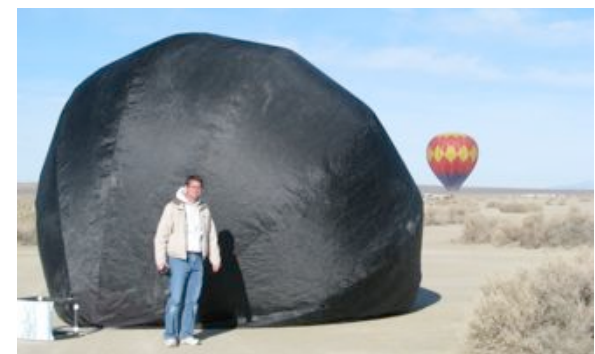
Successful aerial deployment and inflation test on 4.5 m balloon (300-400 meter altitude)
